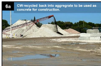
Figure 4-2. The collection and recycling process of concrete washout using a specifically fabricated collection container. The collection to recycling process is shown starting with photo 1 to photos 6a/6b.
